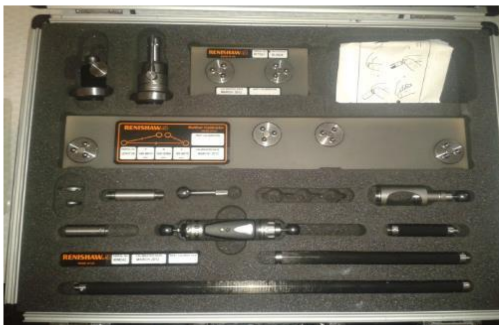
c. Qualitative analysis of the geometry of the machine tool axes, performed with the help of the BallBar kit Renishaw QC20.
